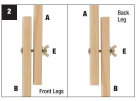
Place two Bottom Legs **(B)** *in front of* the outer Top Legs **(A)** and loosely connect each leg using the Leg Bolt Assembly **(E)**. Place the third Bottom Leg *behind* the center Top Leg **(A)** and loosely connect them using the remaining Leg Bolt Assembly **(E)**.
