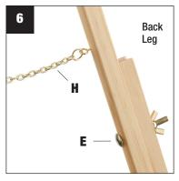
At the other end of the Leg Chain **(H)**, push and turn the screw eye into the wood of the center back leg just above the Leg Bolt Assembly **(E)**.
