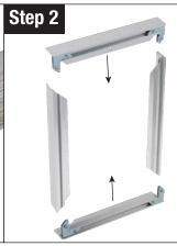
Slide each frame segment with brackets into the adjacent segments and loosely tighten the slotted screws.
