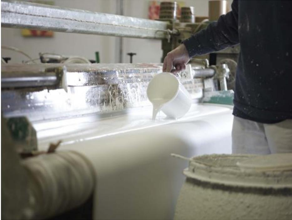
Because this primer and coating are water-based, these canvases can be dried in the dry-air oven, where the water can evaporate more quickly.
