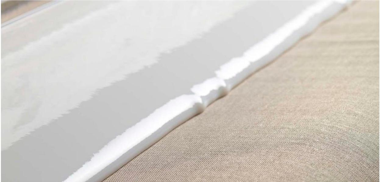
We always apply 2 layers of synthetic adhesive. After each layer the canvas is dried in a warm-air oven.
