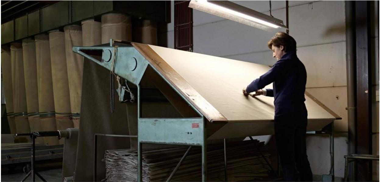
When the fabric arrives at Claessens, it is first checked with great care for any weaving faults. Abnormally thick threads and any unevenness are scrupulously removed.
