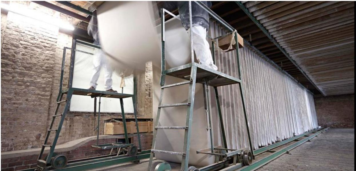
After the 1st primer, the canvas is placed in a drying room for three days where it air-dries naturally. Double-primed canvases undergo the same process once again. When the final coating is applied, the canvas then has to go back into the drying room for a further ten days.
